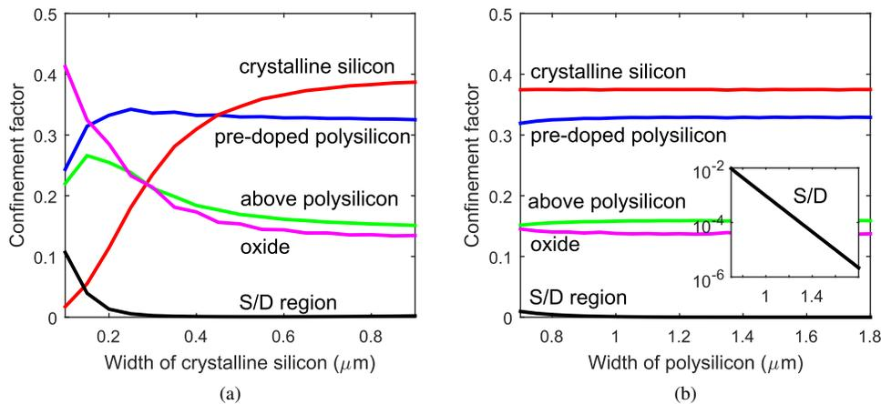
Fig. 3. (a) Crystalline silicon ridge width of 600 nm keep confinement factors in S/D region small. Additionally, it also reduce confinement factor above polysilicon. (b) Central polysilicon width of 1.6  $\mu\text{m}$  reduces the confinement in S/D region to below 0.1%.
