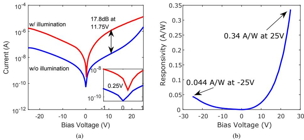
Fig. 6. (a) I-V curves of the resonant photodetector without and with  $40 \mu\text{W}$  light launched into the waveguide. The inset shows a close-up of the I-V curve near the 0 V bias showing an open-circuit voltage. (b) Responsivity at 1550 nm versus bias voltage with  $40 \mu\text{W}$  optical power into the device.
