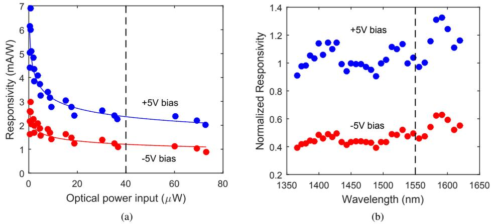
Fig. 7. (a) Responsivity of the resonant photodetector as a function of the optical power entering the resonator at 1570 nm under 5 V reverse (red curve) and forward (blue curve) bias. (b) Responsivity of the photodetector from 1360 nm to 1630 nm for  $20\mu\text{W}$  optical power entering the resonator normalized to responsivity at 1550 nm with 5 V forward bias.
