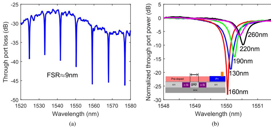
Fig. 5. (a) Resonance is achieved from 1520 nm to 1580 nm. The FSR is around 9 nm. (b) Highest extinction is obtained at gap size of 160 nm. Gap sizes between 130 nm and 190 nm production extinction more than 10 dB.
