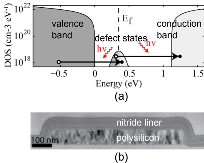
Fig. 1. (a) Polysilicon density of states (DOS) showing defect states in polysilicon assisting sub-bandgap photon absorption and electron-hole pairs generation [22]. (b) Transmission electron micrograph of gate polysilicon showing the grain structure and the surface roughness [21].
