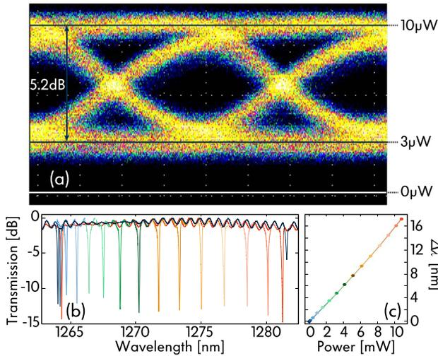
Fig. 3. (a) 5 Gbps optical eye diagram with 5.2 dB modulation depth in response to drive voltage swing from  $-3$  to  $+0.6$  V (at the device terminals), (b) thermal tuning of the modulated resonance across a full FSR (efficiency: 291 GHz/mW), and (c) linear resonance tuning versus heater power.
