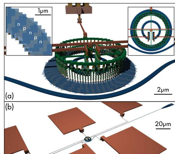
Fig. 1. (a) Layout of monolithically integrated modulator showing spoked contacts, radial *p-n* junctions, mode-selective waveguide coupler, and back-end metal stackup (left inset, contacts and lateral junctions; right inset, top view showing central heater). (b) Zoom-out: driver and heater contact pads and input grating coupler.
