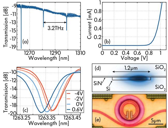
Fig. 2. (a) Optical transmission spectral response with single transverse-mode operation evident (FSR = 3.2 THz, extinction near 1260 nm is >10 dB), (b) device I-V curve, (c) resonant optical response at DC bias voltages from  $-4$  to  $+0.6$  V, (d) calculated cross-sectional mode profile (the waveguiding body silicon and the nitride liner layer above it are outlined), and (e) optical micrograph of the device taken from below after removal of the handle Si wafer.
